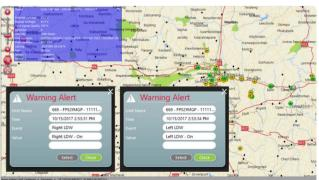
Install identification devices (Dallas, RFID cards, numeric keypads, etc.) to control access to your vehicles. Fleet managers are alerted of abnormal activity and are capable of remote vehicle mobilization or immobilization.
